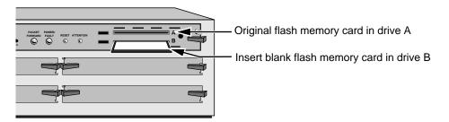
2 Format the blank flash memory card in drive B by entering: FORMAT b:
